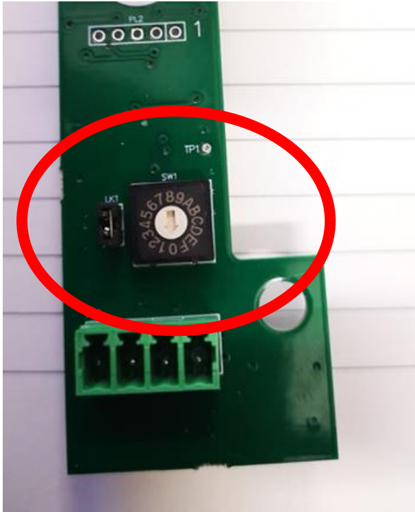
Figure 1 - Rotary switch to select Maximum current rating
